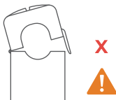
Incorrect CT Installation
